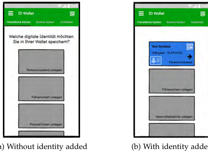
Figure 11: Main View of the low-fidelity prototype, also showing all identities in a tabbed view. The option to add a new identity is integrated into the main view.
